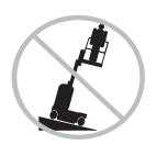
Do not raise the platform unless the machine is on a firm, level surface.
